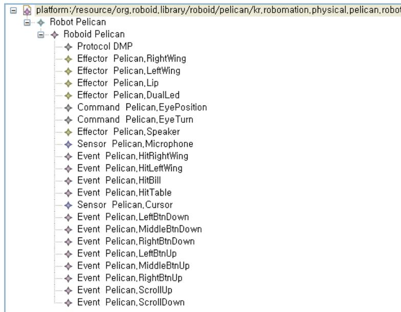
Figure 2.3 Pelican model (`kr.robomation.physical.pelican.robot` file in folder `roboid/pelican`)
